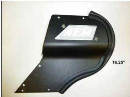
13. Install the AEM® logo into the heat shield and secure with the provided hardware. Install the edge trim onto the heat shield as shown.
