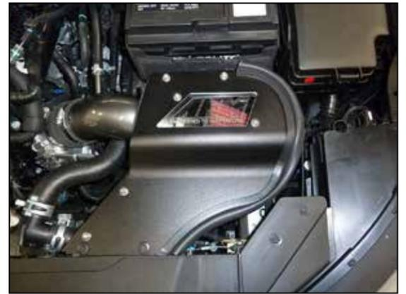
15. Install the lid onto the heat shield and secure with the provided hardware.
