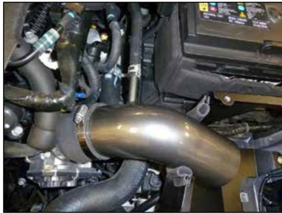
11. Install the AEM® intake tube into the coupler and connect the crank case vent hose and secure with the factory clamp.
