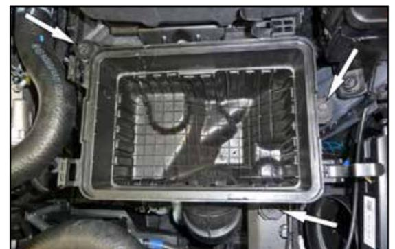
5. Remove the three bolts that secure lower air filter housing and then remove the lower air filter housing from the vehicle.
