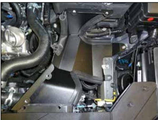
10. Install the heat shield assembly into the vehicle and secure with the provided hardware.
